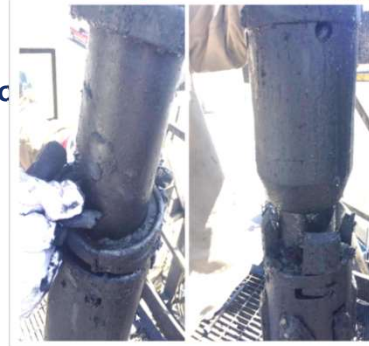
Zone 3 Packer. Rings and slips caused significant drag
