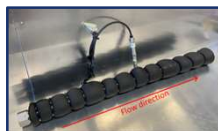
Detachable test section (0.83" I.D.)
