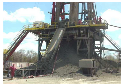
Massive solids production from a well
