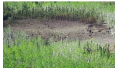
Steam injection that erupted at the surface.
