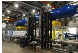
Full scale subsea jumper with WGPM being tested at NEL
