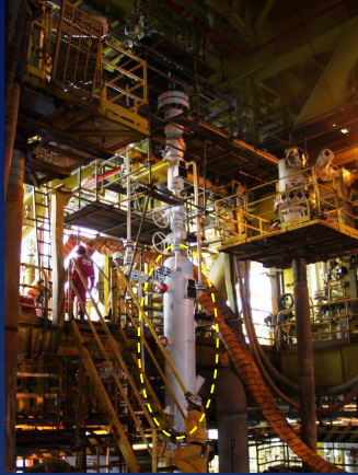
Wellhead Desander Acc. ASME 1500#, 600 liter Malaysia 2011
