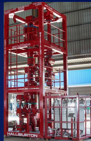
DNV Transport (Closed) Dewatering Bin Saudi Arabia 2013
