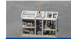
Subsea Seawater Treatment Field Trial (Congo)
