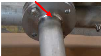
Part after pickling and passivation
