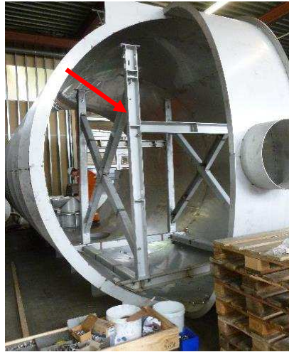
Support beams inside of the vessel
