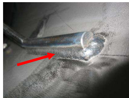
Part after pickling and passivation
