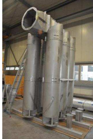
Inlet cyclones ready for final inspection
