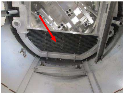
Installation vanepack assembly – vertical vessel
