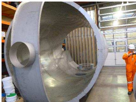
Horizontal vessel (304 stainless steel material)
