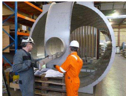
Parts accessibility (fit) thru manway
