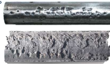
Rod body corrosion pitting
