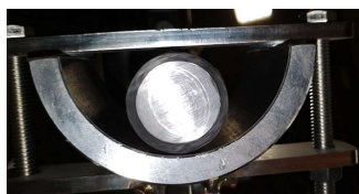
Testing configuration with coated continuous rod and tubing
