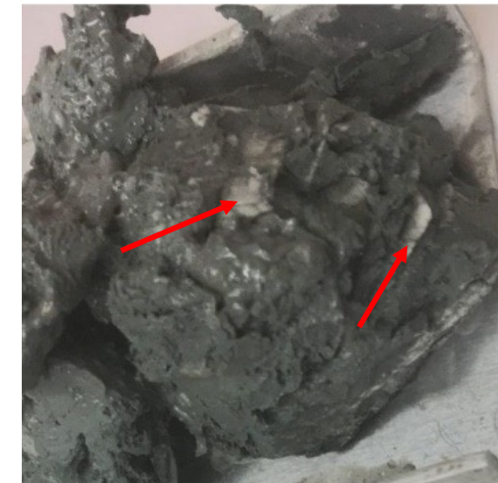
Fracture-filled gas hydrate veins in clay sediment extracted from eastern Qiongdongnan Basin, China
