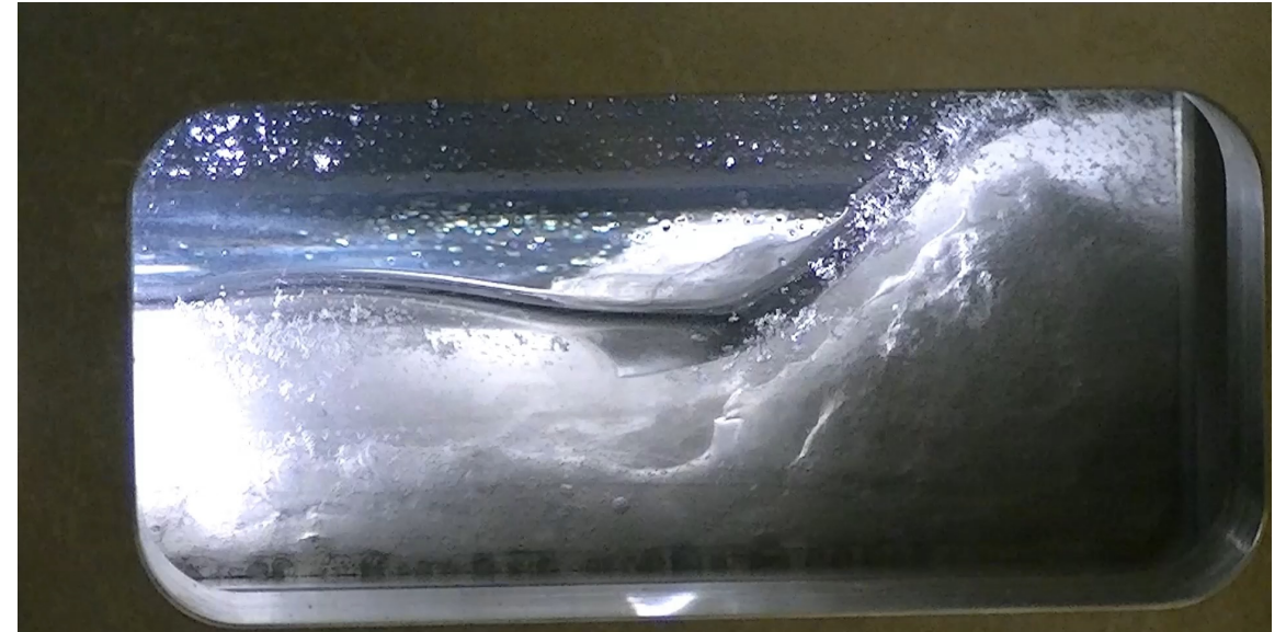
Hydrate deposition on pipe wall
