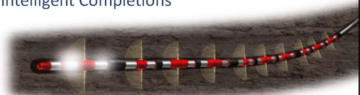
Open hole isolation in multistage fracturing
