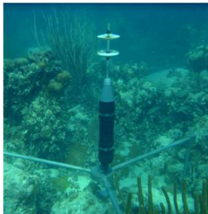
System utilizing differential travel time to measure 3D flow profiles
