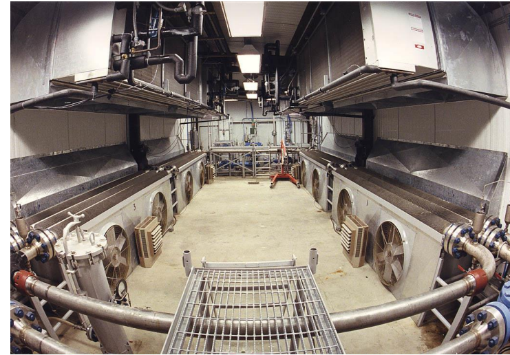
Hydrate test in the XoM Friendswood flowloop
